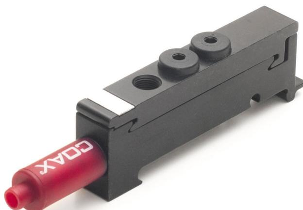
Compact/stackable vacuum pumps are air-driven multistage ejector families, based on COAX® technology, they are equipped with integrated controls and special functions, such as on/off valve, blow-off valve, vacuum switch, energy saving function etc. They are configurable platforms, making it easy to specify the exact control functions needed for the system.
