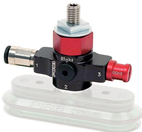
Piab VGS™ – A product design where different suction cups are integrated with vacuum cartridges based on the patented COAX® technology. The “vacuum gripper” makes selection, sizing and installation of a vacuum system easier. With a VGS™ you will enjoy the benefits of a more cost-efficient and reliable decentralized vacuum system. It has a low weight at 25–39 g.
