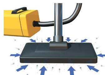
*A vacuum cleaner does not suck. Air and dust are pressed into the vacuum cleaner by the surrounding higher atmospheric pressure.*
