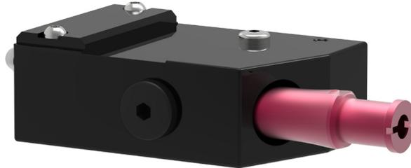
This is a product design where different suction cups can be integrated with vacuum cartridges based on the patented COAX® technology. The “vacuum gripper” makes selection, sizing and installation of a vacuum system easier. With a VGS™ you will enjoy the benefits of a more cost-efficient and reliable decentralized vacuum system. The VGS™ is compatible with any suction cup with G3/8” male fitting. It has a low weight at 204–340 g.
