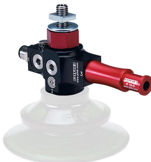
Piab VGS™ – A product design where different suction cups are integrated with vacuum cartridges based on the patented COAX® technology. The “vacuum gripper” makes selection, sizing and installation of a vacuum system easier. With a VGS™ you will enjoy the benefits of a more cost-efficient and reliable decentralized vacuum system. It has a low weight at 111–340 g.
