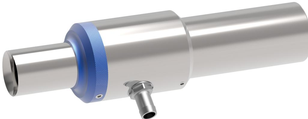
This is a compact ejector pump which is normally used when a large flow with low vacuum is desired. The air consumption and capacity can be adjusted. Small amounts of material and contaminants can be conveyed. This product is available in stainless steel or aluminium. When it is fitted with an insert, the ejector changes characteristics providing higher vacuum at lower flow. It is delivered with a 3/8" hose nipple for the compressed air connection.
