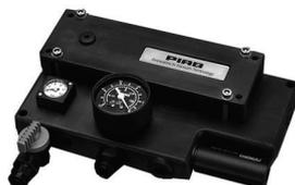
This vacuum pump is tailor-made for laboratory applications, such as degassing, vacuum filtering, gel drying and rotation evaporation. It can achieve high vacuum levels to 20 mbar abs. with a maximum vacuum flow of 9 m<sup>3</sup>/h. There is no risk for “back draft” which can cause damaged test samples. Its low noise level, easy installation and maintenance is widely appreciated.
