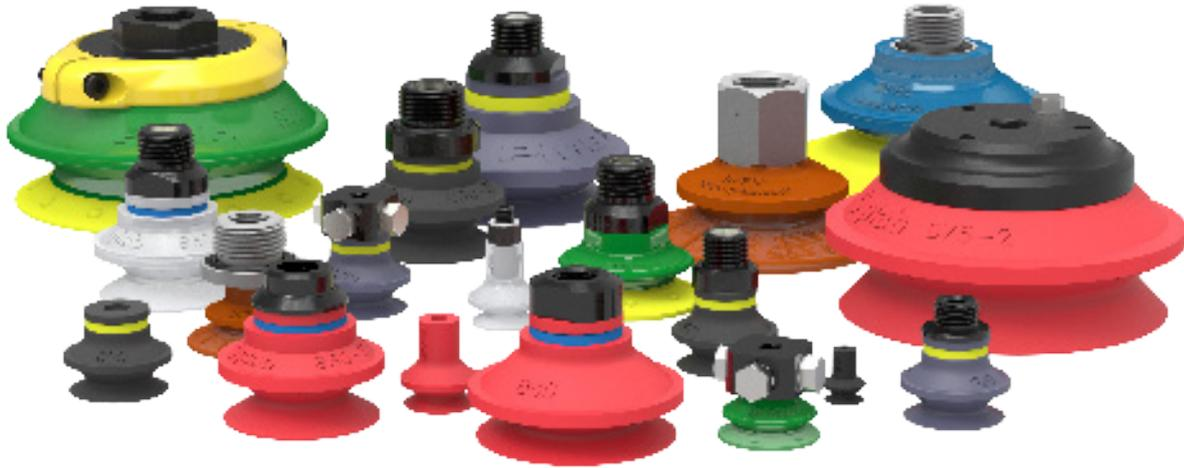
The bellows family is suitable for height differences and slightly uneven or curved surfaces. Several short bellows cups in one lifting device can handle objects with height differences and varying shapes. The bellows also provide a slight lifting movement to separate thin items. This family is available, among other material in FDA compliant material, or the durable DURAFLEX® as Mark Free or even for oily surfaces.
