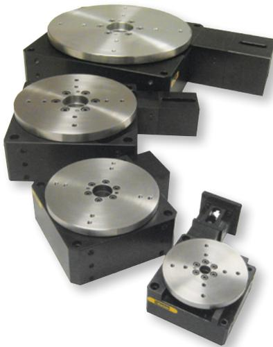
The RM Series offers high load capacity in a compact package. These rotary stages utilize a precision worm gear with the worm “flexed” against the gear to ensure a proper mesh. This feature provides an auto anti-backlash calibration with smooth motion. Additionally, the rotary stages incorporate an oversized preloaded cross roller bearing, offering exceptional stiffness and high normal and moment load capacity.
