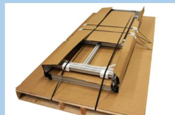
Profiles are cut and machined to order, fasteners and accessories are included based on a parts list, and the entire order is packaged and shipped for final assembly at your location.
