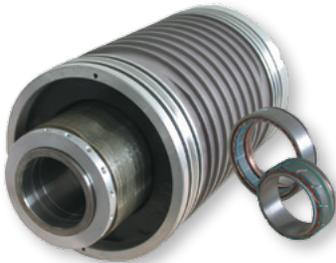
The HW servomotors are water-cooled brushless synchronous motors delivered as individual components (rotor, stator and resolver) to make a complete spindle unit. These motors are driven by Compax3 Series servo drives.
