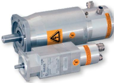
The EX Servo motors are designed to function in Category II, Group II explosive atmospheres in respect to the EN 50014 standard. These servo motors are certified according to directive ATEX 94/9/CE and are available in a Gas or Gas-Dust version. The motors differ in that the Gas-Dust version is equipped with a special lip seal on the customer end shaft.
