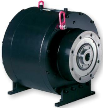
The torque motor is a permanent magnet brushless motor, optimized to operate at low speeds. It is particularly suitable for direct drive applications requiring high torque capabilities at low speeds.
