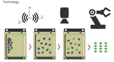
Parts are spread homogeneously on the feeder surface and can even be systematically oriented in many cases by using intelligent vibration patterns in combination with a structured plate. Entire part families can thus be handled with a single feeder, making the system highly future-proof.
