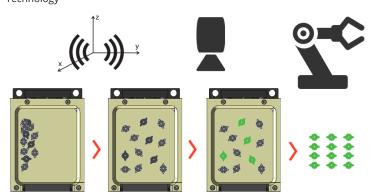
Parts are spread homogeneously on the feeder surface and can even be systematically oriented in many cases by using intelligent vibration patterns in combination with a structured plate. Entire part families can thus be handled with a single feeder, making the system highly future-proof.
