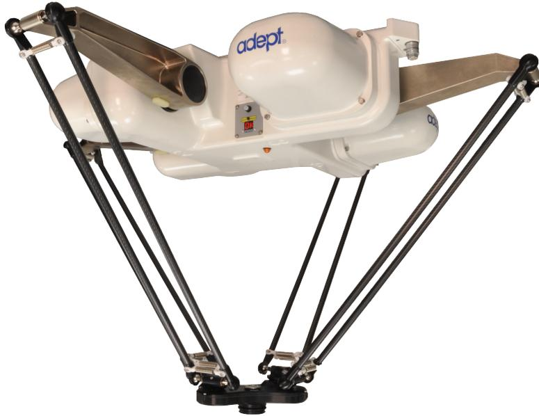
The Quattro™ s650HS is the only high-speed parallel robot in the world that has been USDA-accepted for meat and poultry processing. The patented four-arm design, advanced control algorithms, and large work envelope make the Adept Quattro the ideal overhead-mount robot for smooth motion, high-throughput applications. The Adept Quattro is powered by ultra-compact controls and embedded amplifiers, which reduces the cycle time and improves footprint efficiency.
